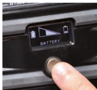
OLED multifunctional display
