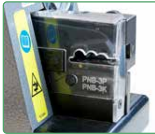
PNB-3P detail of the crimping zone.
